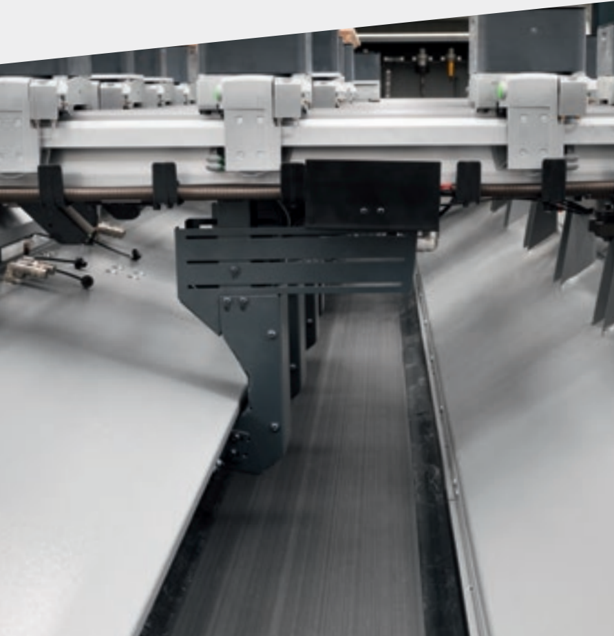
Motorised conveyor belt for the removal of chips and waste.
