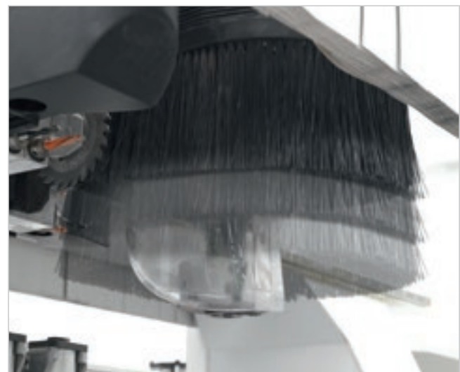
Adjustable suction hood with 8 settings (for 4 axes) and 12 setting (for 5 axes).
